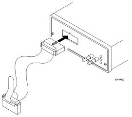
**4** Plug the keyed end of the cable (pin 12 is blocked) into the EJTAG debug port on the target system.
