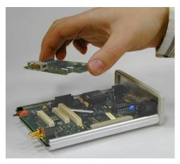
Do not turn on power to the emulation probe when no target board adapter is installed.
